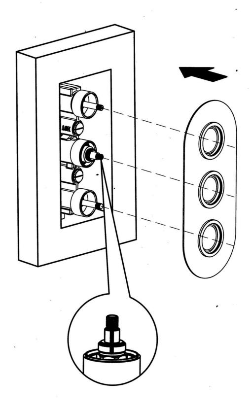
3. Check if the marking line of the thermostatic cartridge are aligned, and then put on the cover plate.
