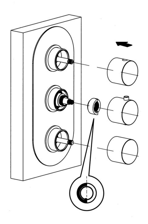
4.Install the thermo stop-ring, thermo handle, flow handle.
