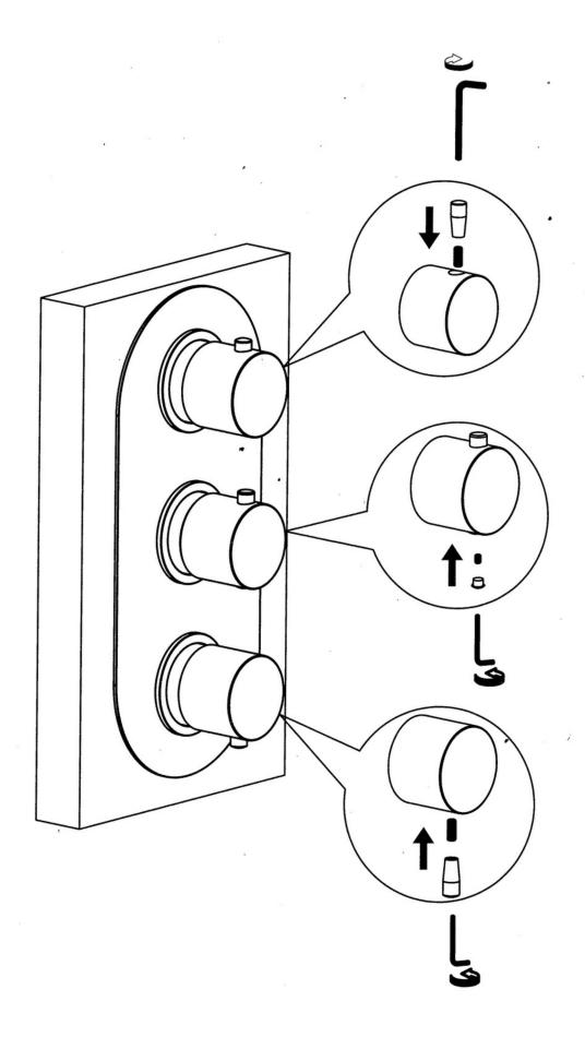
5. Tighten all the handle grubscrews with Allen key.
