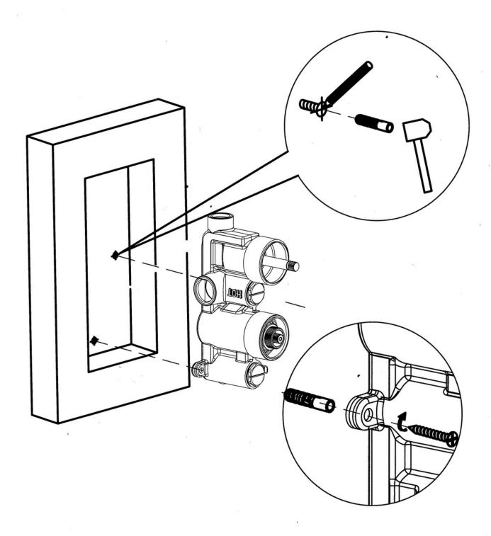
1.Determine the mounting position for the valve, refer to installation dimension drawings, reserve the recess in the wall in which to mount the valve, the depth of the recess should be min 72mm, max 82mm. Fix the valve with tapping screws and wall plugs.
