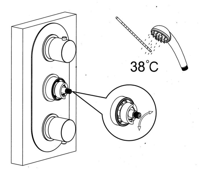
7.If there is a large deviation of the outlet water temperature from the default 38°C (deviation of ±2 °C is the normal range), remove the thermo handle, fine-tune the handle left and right to adjust the water temperature to 38±2°C, and then reinstall the thermo handle.
